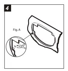
Cut and remove the shaded portion of the sub-dash lip. (see Fig. A)
